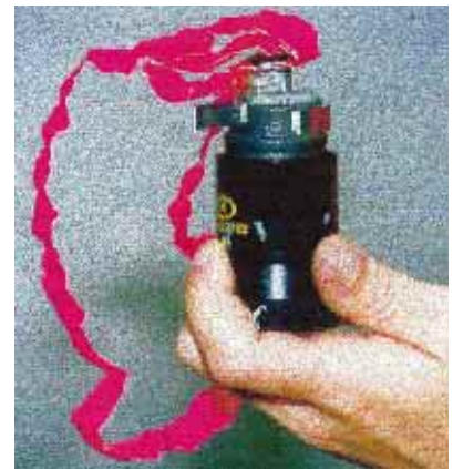
[K] French Submunition OGR F1 equipped with a pink ribbon. (Photo: EC, NEDEX)
